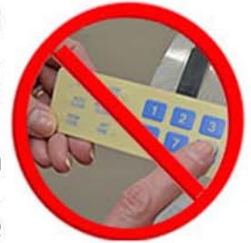
Keep part flat on a solid surface when pressing a button on the switch.
